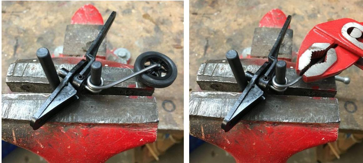
*To adjust the tail wheel, use two metal rod`s (may be two 5.5 mm driller). Use a long claw and adjust the tail wheel.*
